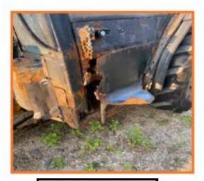
The 1998 Colpron Landini is experiencing significant rusting and pitting on the frame and plow attachment and severe mechanical problems.
