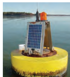
FIGURE 5.1 Datasonde buoy deployed in Great Bay
