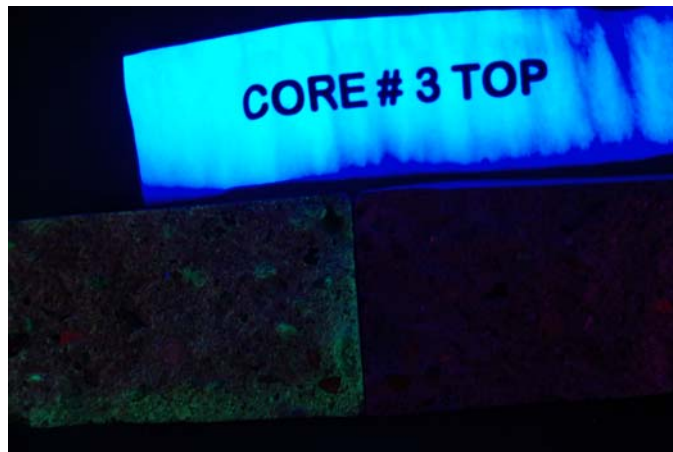
Figure 27 Core #3 Top tensile sample treated with Uranyl acetate dihydrate (left side) under normal light (top) and ultra violet light (bottom)
