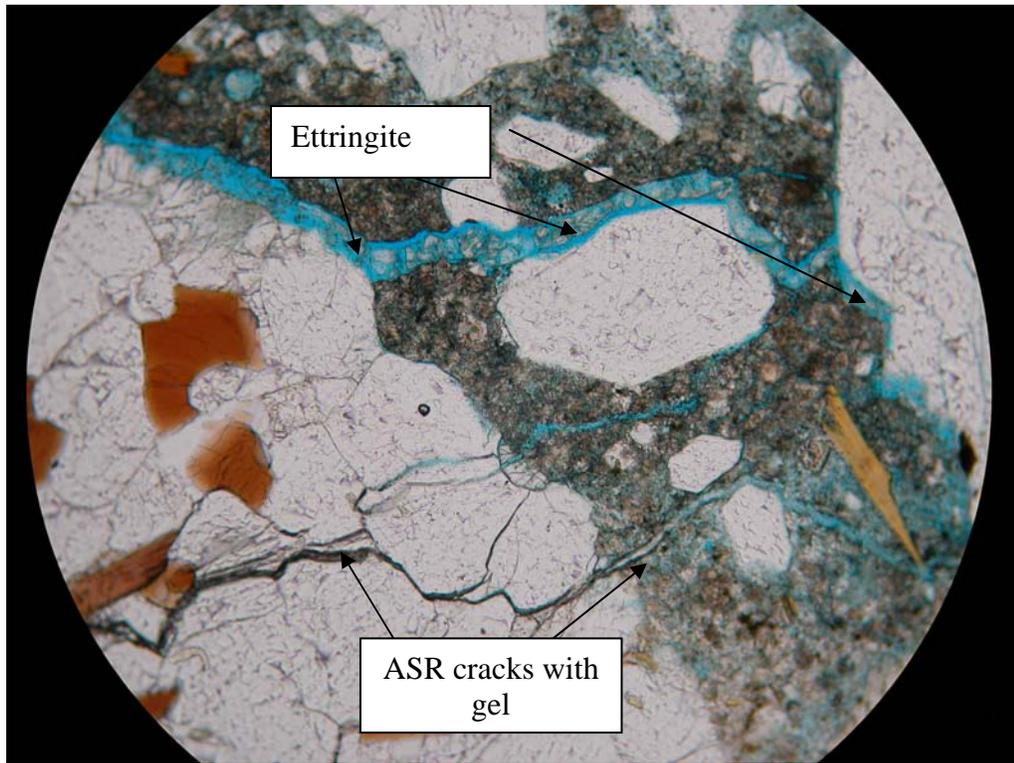
Figure 41 Core 13 horizontal section showing ASR and Ettringite
