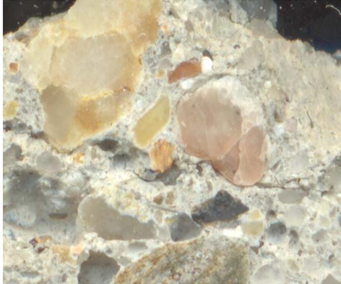
Figure 5 Section A close up of Figure 4 core #5
