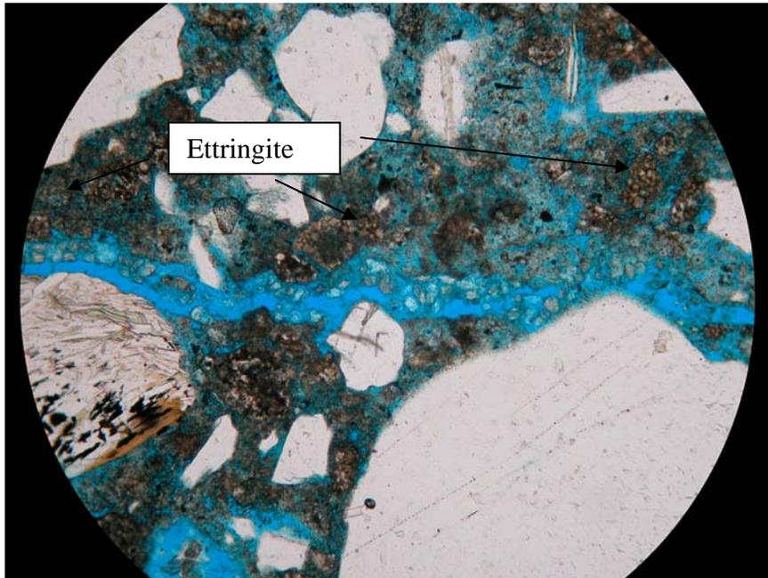
Figure 36 Core 13 horizontal section showing secondary ettringite
