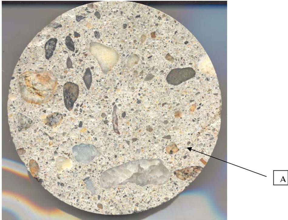
Figure 1 Core # 1 polished surface of top
