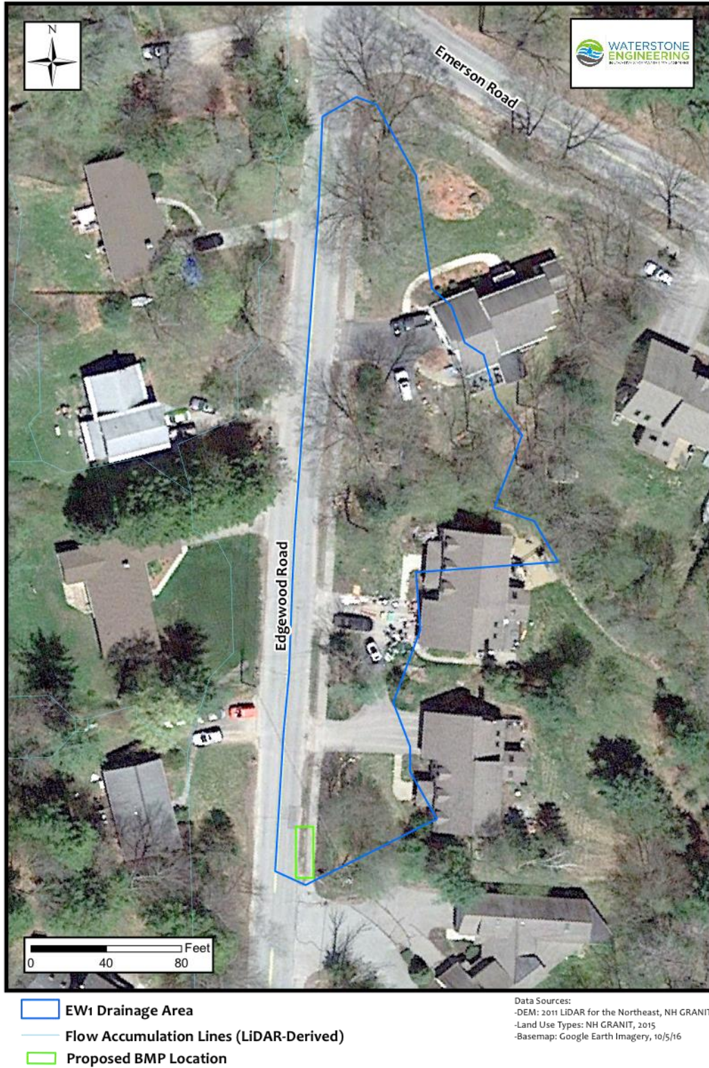
Figure 16 – Edgewood Road BMP 'EW1' Detailed Location and Drainage Area
