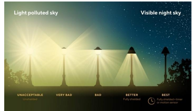
Figure 4: A chart depicting four levels of shielding for outdoor lights, plus one light that is turned off. DarkSky International
