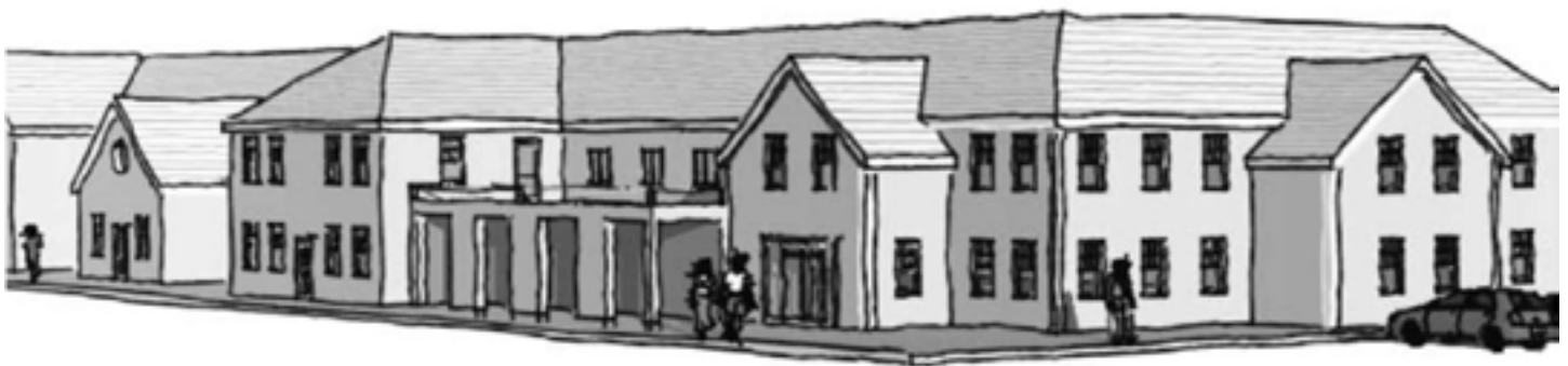
As shown in this sketch, lower roof eaves on attached masses reduce the apparent scale of the building.
