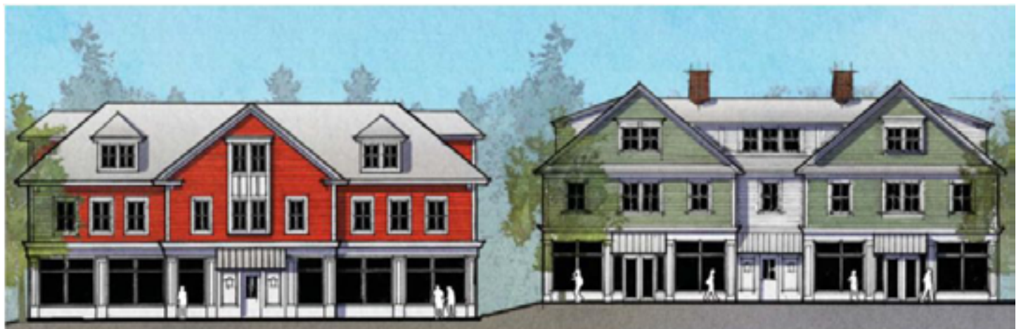
A complex of smaller scale buildings is preferable to a single large structure because the varied massing provides visual interest and human scale.
