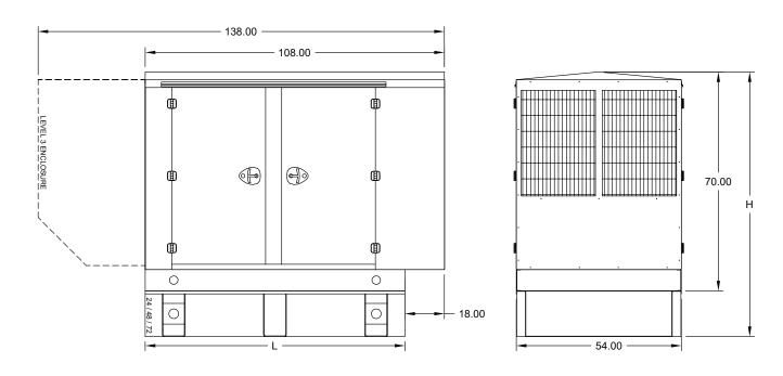
All enclosure models are 200 MPH wind rating certified in accordance with IBC2018 and ASCE/SEI 7-16 standards.
