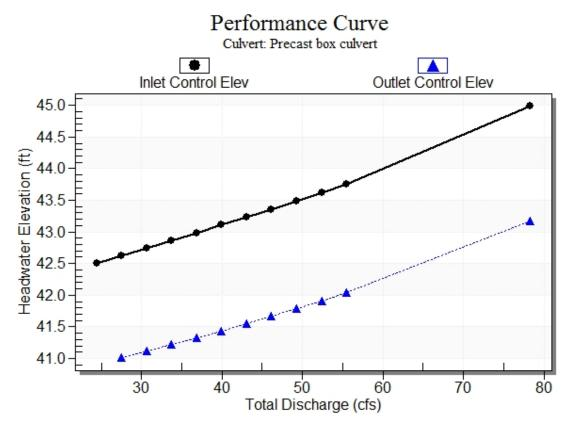
**Culvert Performance Curve Plot: Precast box culvert**
