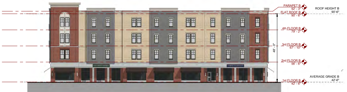
C1 EXTERIOR ELEVATION - "B" SOUTH SCALE: 1/16" = 1'-0"
