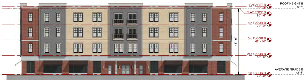
B1 EXTERIOR ELEVATION - "B" NORTH SCALE: 1/16" = 1'-0"
