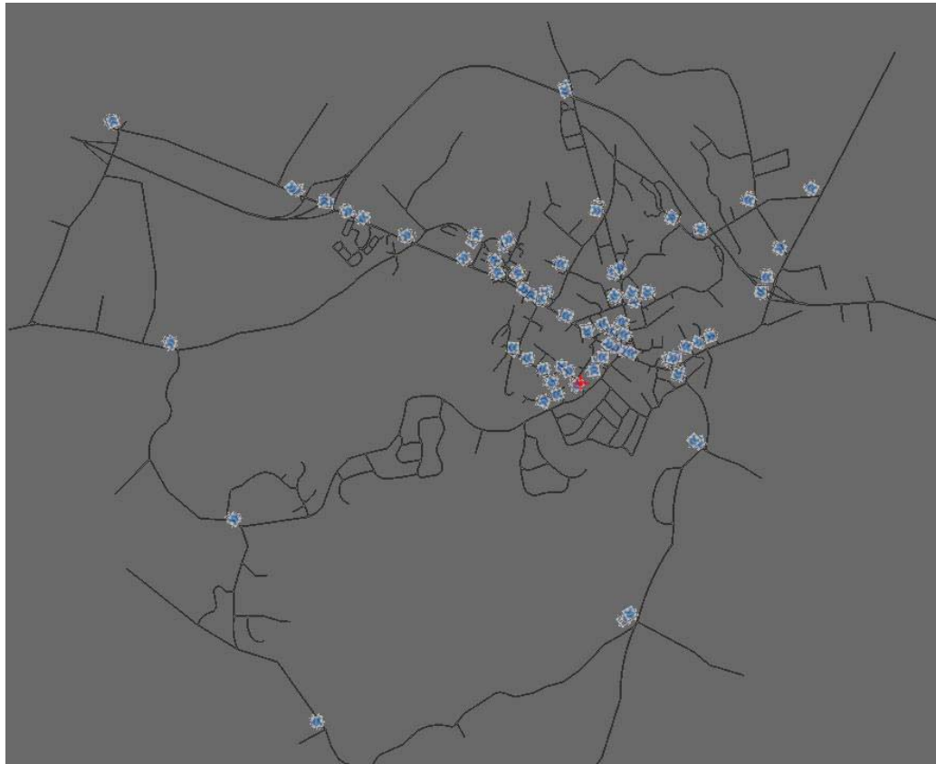
Figure 7: Paramics “Estimator” Interface Showing Locations of Calibration Count Set in Model
