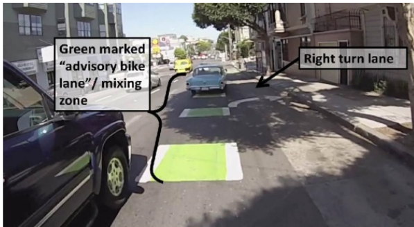
Turning Zone with Unrestricted Entry and Through Bike Lane (TBL) Photo from survey (shown): Oak St. and Divisadero St. Video Location(s): Oak St. and Divisadero St.
